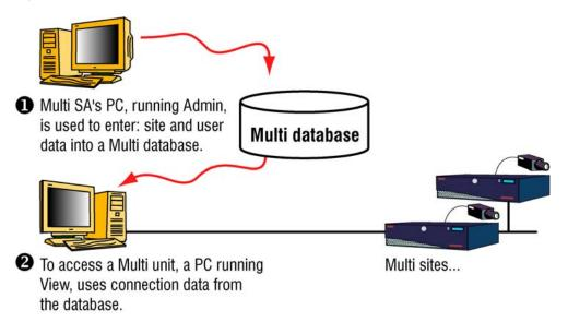
When a unit operator logs on to View, a local copy of data about the operator and the sites he may access, is made from the Multi db to the PC.
